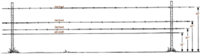
4-strand Barbed Wire with Bottom Smooth Wire Figure: MT-FWP
